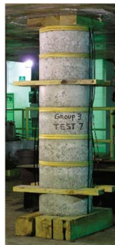
Figure 3 - CribPac (Group 3), 1 1/2 inch plywood separators
