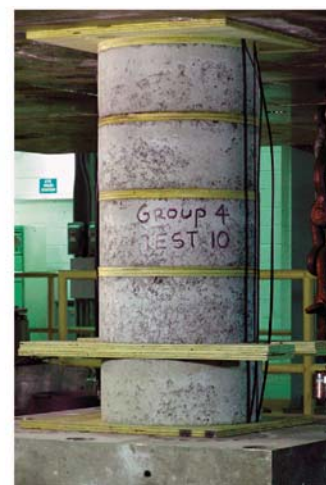
Figure 4 - CribPac (Group 4), 1 inch plywood separators
