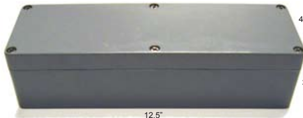
Fixed Node - Small, rugged structure with no external antennas or power wires
