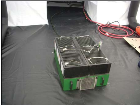
A replicated, fully functional carbon dioxide scrubber is stored in the skid.
