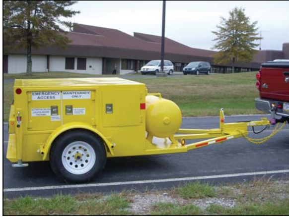
Lightweight, trailer mounted and road worthy, the Fresh Air Bay Training Unit can be towed to mine site locations
