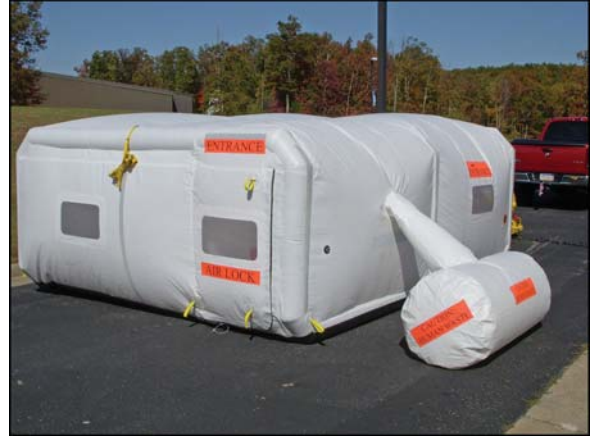
The Fresh Air Bay Training Unit Tent is a replica of the production units, including a fully functional airlock entry chamber and an external waste disposal bag
