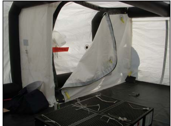
Airlock entry chamber complete with functioning purge air controls
