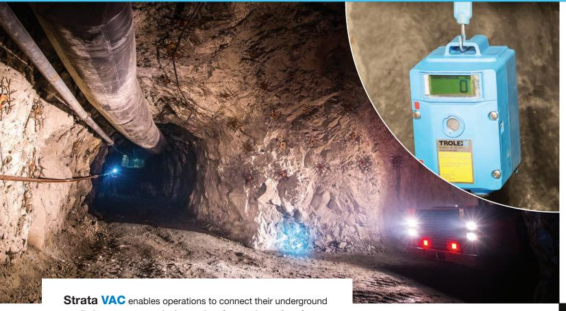
ventilation system to a single user interface at the surface for automation and remote control. The fan automation is based on pre-selected environmental variables and adjusts the fan speeds and turns fans on and off automatically as needed. By automating these processes, unnecessary activity and usage is eliminated which results in decreased energy costs.
