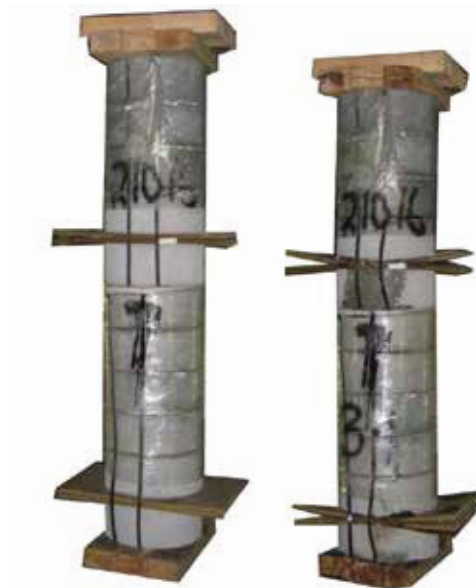
Cribpac yielding under load
