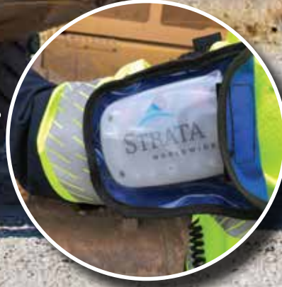
Belt-, arm- or hard hat-worn personal alarm device alerts worker of potential danger
