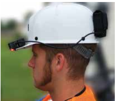
Hard Hat Mounted PAD with Warning Module
