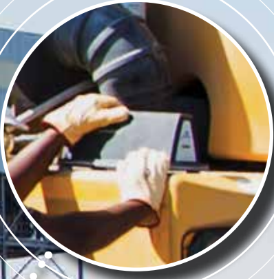
Proximity Generators mounted on machinery create electromagnetic field(s) around entire vehicle.
