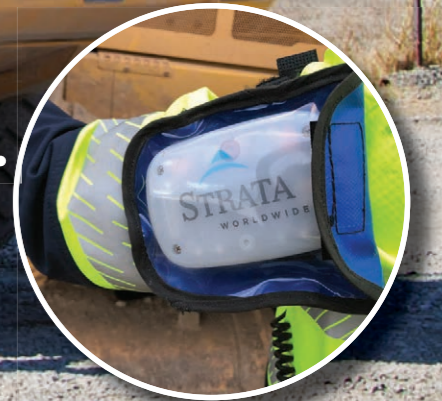
Belt, arm, vest or hard hat worn personal alarm device (PAD) alerts worker of potential danger
